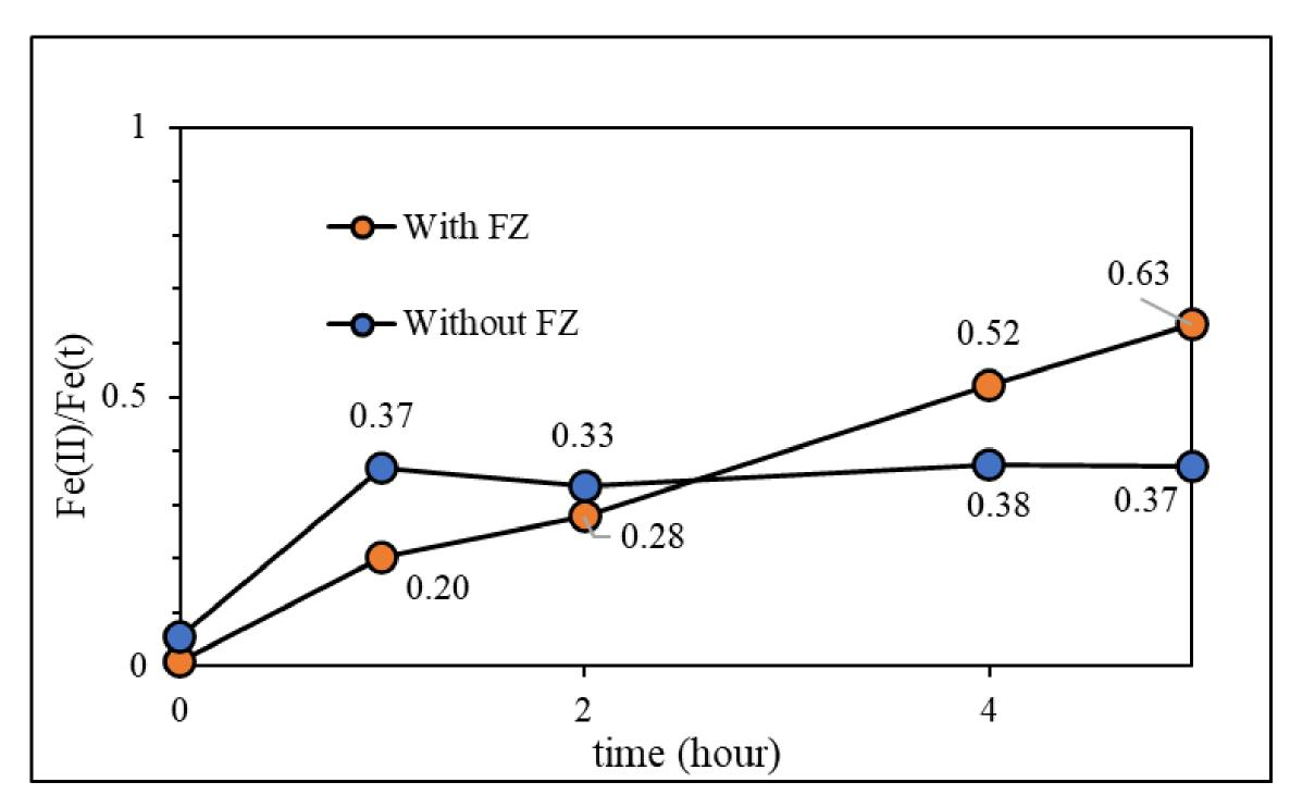
The effect of FZ. Comparison of Fe(II) production with and without FZ present during UV-B exposure.
