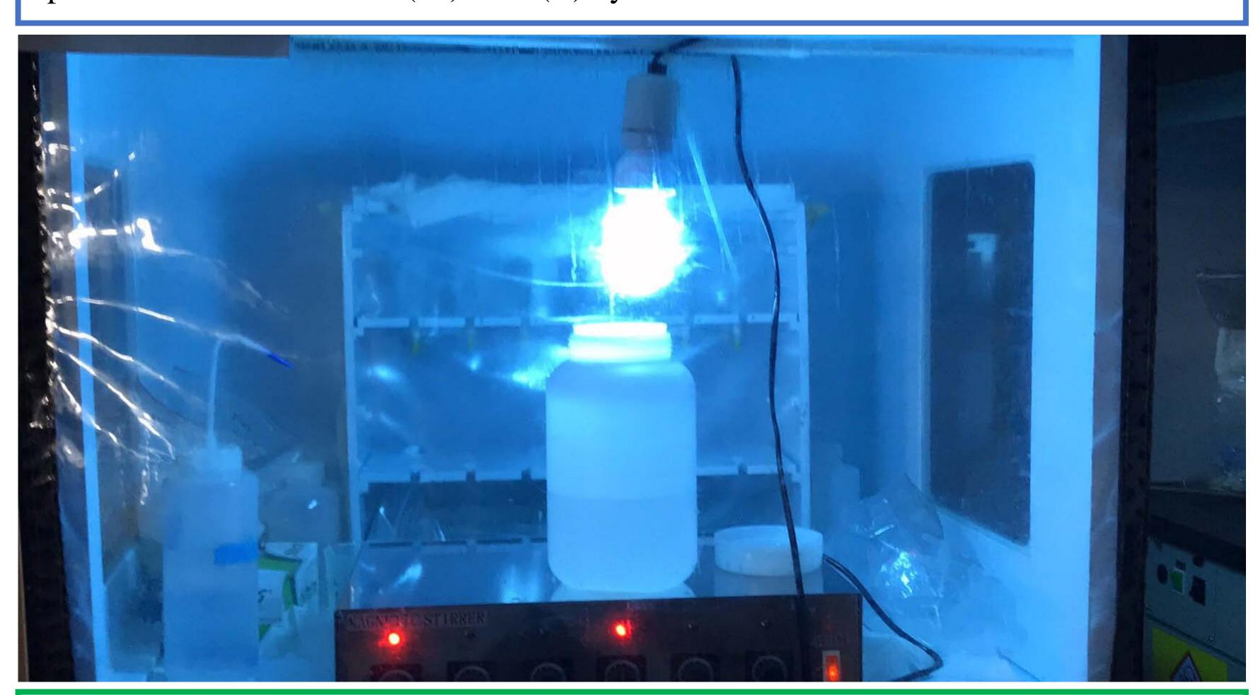
**UV exposure setup:** Experiments were carried out in a HEPA controlled chamber. Samples in 2 liter PE bottles were mixed by stirrer and collected and transferred to 50 mL polypropylene tubes at hr 0, 1, 2, 4, and 5. The collected samples were then measured by spectrophotometer after the treatment shown on the right.
