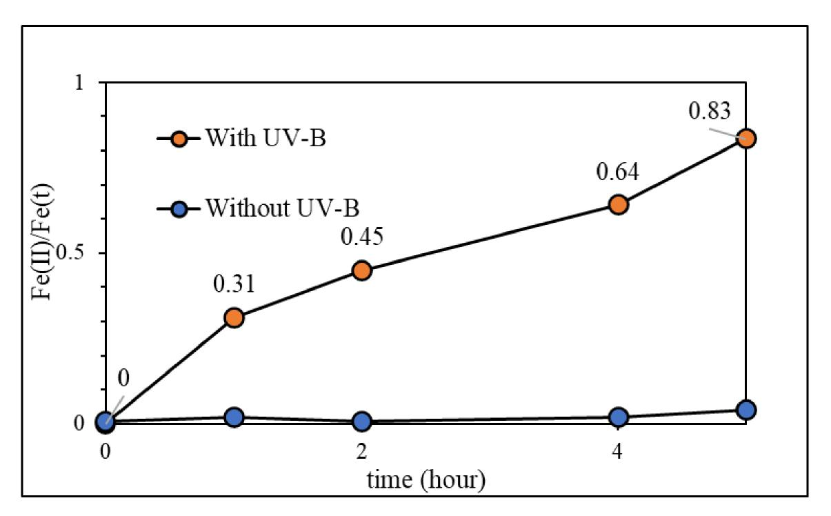
The reduction of Fe(III) by UV-B. The results show that UV-B exposure significantly increased the production of Fe(II) over 5 hr.
